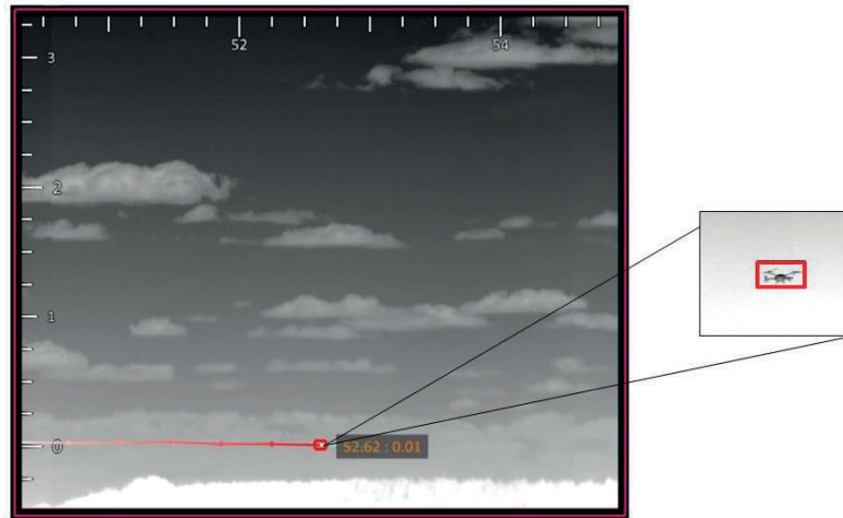
Figure 2 - A Cyclope screenshot shows a small UAV being detected and tracked
