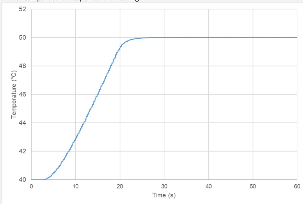
Figure 3. Regulation curve of a high stable blackbody
