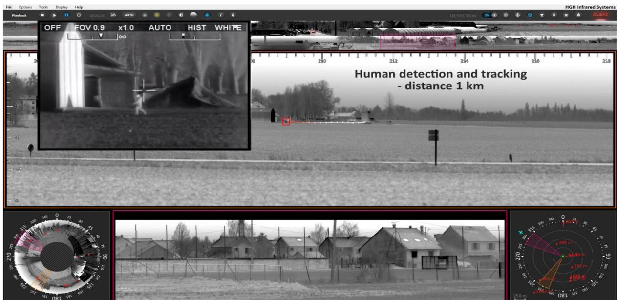
**Figure 3** - This Cyclope screenshot shows a standard PTZ plugin tracking a human through a field identified by Spynel for up-close identification. The red box at the top alerts the operator that a target is detected and automatically tracks.
