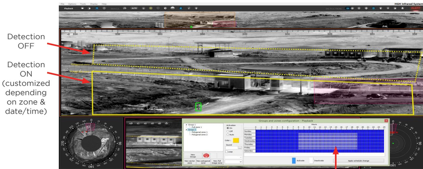
**Figure 4** - This Cyclope screenshot shows a completely customized interface as per an operator’s preferences: 360° strip window shows full surrounding at the top of the screen; alarm activation set to trigger according to specific date/time; sound and visual alarms output; list of possible target classifications; and two different detection zones based on date and times-one activated, the other turned off.
